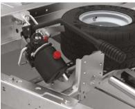
**O** Hydraulic tilt-bed Powerful self-contained hydraulic ram powers the tilt-bed operation. Choose your ideal loading ramp solution to go with it.
