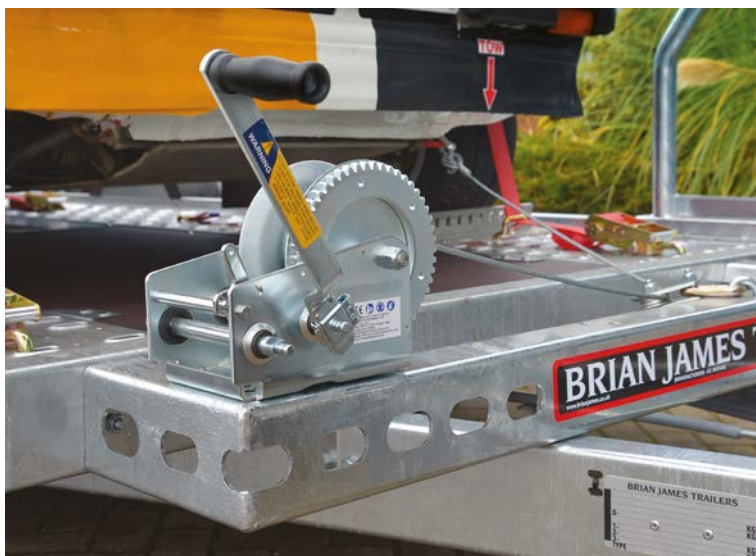
○ Manual winch + 3 point adjustable pull positions.
